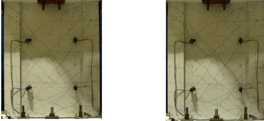
Figure 6. Crack pattern of the test specimen: Left: at the end of GM1; and Right: at the end of GM2.
