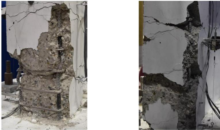
Figure 8. Bar buckling and loose broken concrete of the RC wall after the pushover test.
